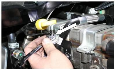
12.Remove the EGR coolant hose from the cylinder head to the cooler. (All bolts should be already removed) the hose is held in by orings. Remaining coolant will drip out.
