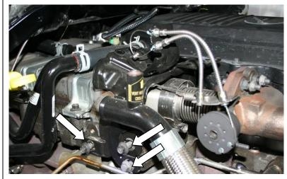
6.Remove the three bolts for the stepper motor bracket (10 mm) socket and prop the bracket on the cooler.
