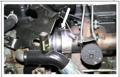
8.Using a (15mm) socket remove the outer nut for the exhaust flange of the flow valve at the manifold.
