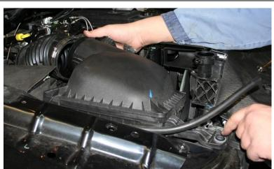
5.Remove the top bolt from the lower heat shield (10mm) then the other two (8mm) bolts to release the lower heat shield.
