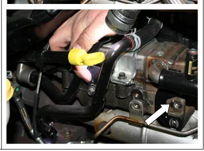
11.Remove the four bolts for the cooler and the nut that holds the transmission dip stick tube in place. Then nudge the tube out of the way to access the nut under the dip stick bracket.
