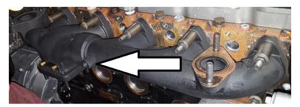
Please note the M12 inverted flare port is for the OEM back pressure sensor.
